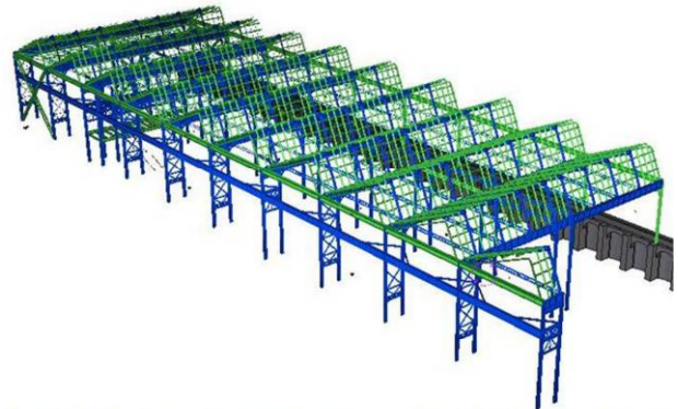
Figure 5: Bim model of the steel existing frame before modifications.
