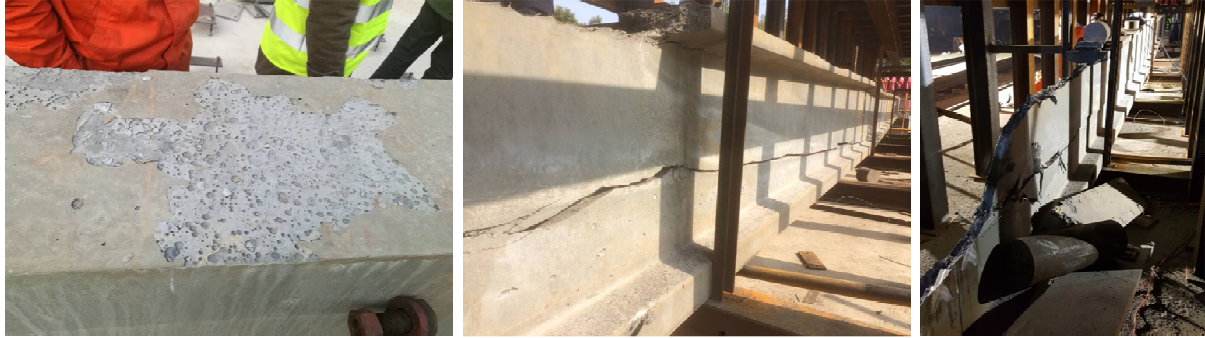
Figure 16 :View of final rupture due to testing process
